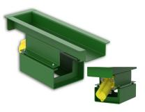
Functionally, there is no benefit to locating the vibrators above, on the side or below the unit. Provided the structure is appropriately designed for the force output of the vibrators and they "sense" each other, either vibrator location can provide satisfactory results.
